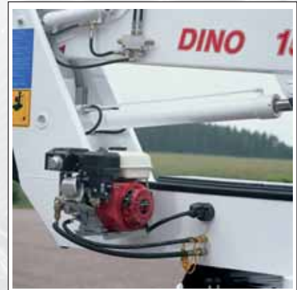
The optional Honda petrol engine provides energy supply wherever electricity is not available.
