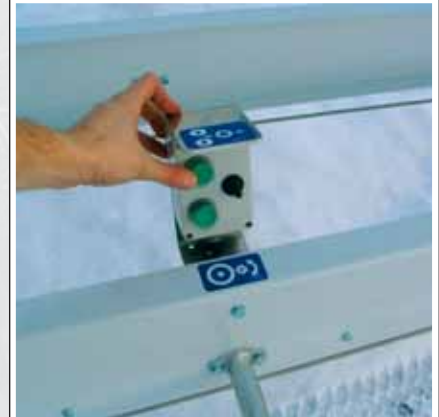
The driving system of the DINO 210XT is operated from the control box which is mounted on the side of the tow bar.
