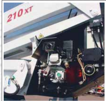
The platform may be powered by mains electricity or petrol engine.
