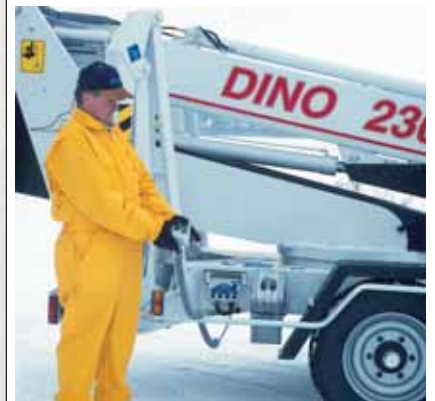
The driving system of the DINO 230T may be operated either with the push buttons on the chassis or with the cable control available as an option.
