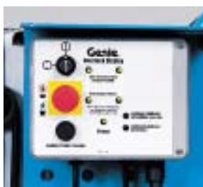
Ground Controls include a low-battery indicator.
