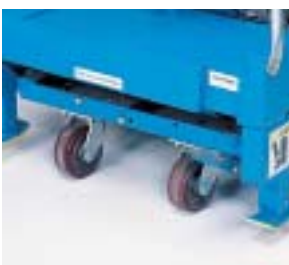
Foot pedal raises the base for easy maneuverability.
