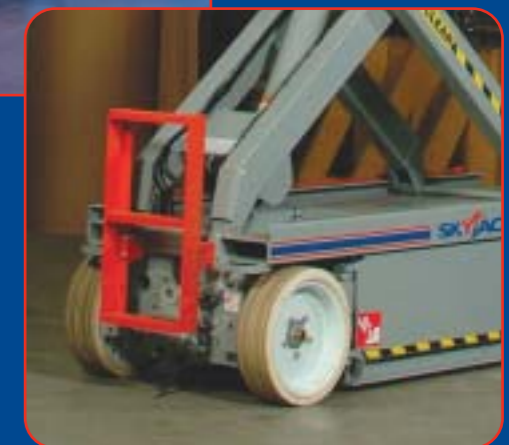
SJIII Conventionals feature variable speed rear wheel hydraulic drive.
