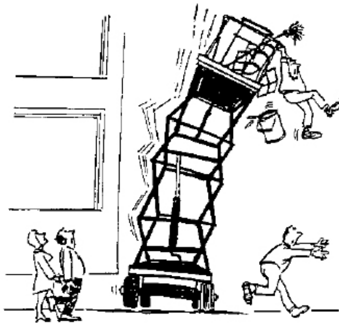
An unevenly distributed load will reduce stability
