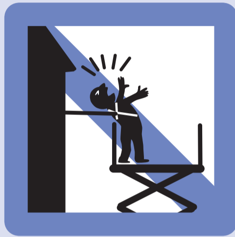
Do NOT attach harness to structure outside the platform
