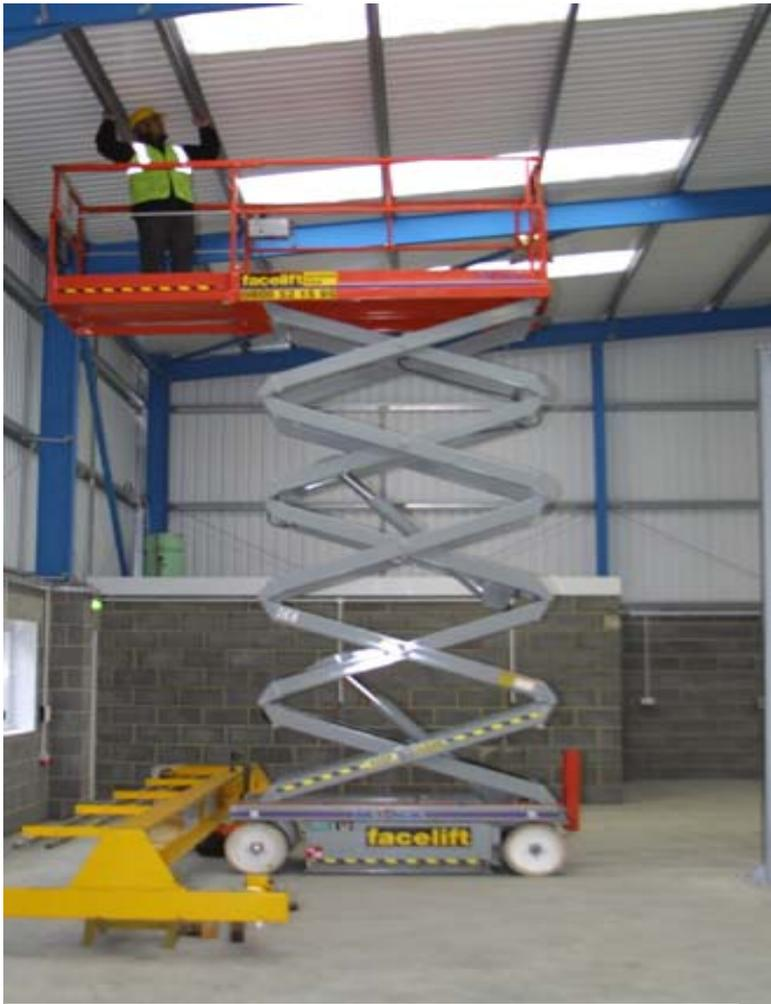
The rollout deck allows a greater working area, idea for warehouse maintenance. Also the added outreach assists when working over obstacles.
