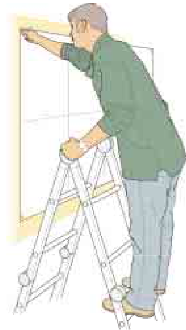
Figure 11 Correct - two clear rungs. Don't work any higher up this type of stepladder
