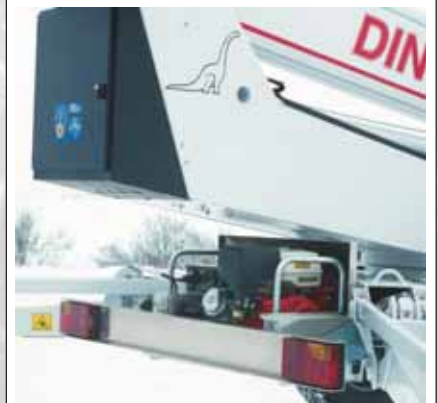
The petrol generator, provided as standard, produces power for both the platform and tools.
