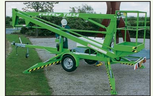
The TM34's manual outriggers are both cost effective and simple to set up.
