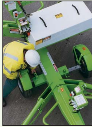
Retractable axles allow the TM34 to pass through a 3ft 6in (1.10m) wide opening.
