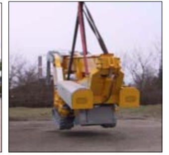
Lifting eyes are fitted.
