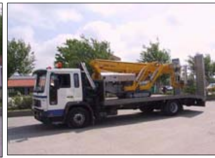
Transport on a truck with a ramp.
