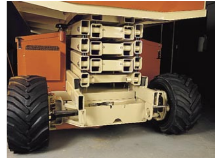
Strengthened Arm Stack for Improved Stack Rigidity
