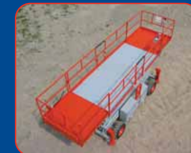
The Full Size Series offers optional dual extension decks increasing platform work area up to 24' (7.3m)
