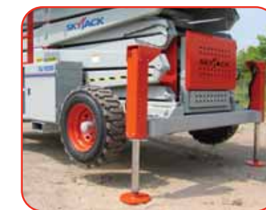
Independent levelling outrigger standard on SJ9250 optional on SJ88XX
