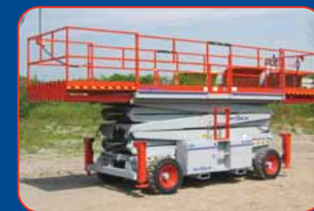
SJ9250 with optional dual power extension decks
