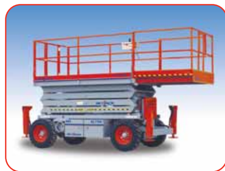
Model: SJ7135 shown with optional independent levelling outriggers.
