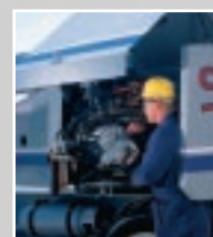
Cabinets swing open and engine pulls out for superior serviceability.
