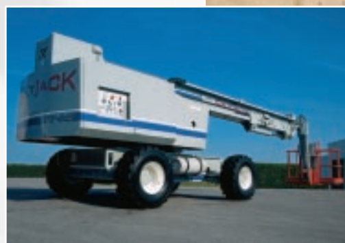
Unique to the SJB-46TK is the pendulum weight mechanism that transfers and distributes weight regardless of boom function or position.
